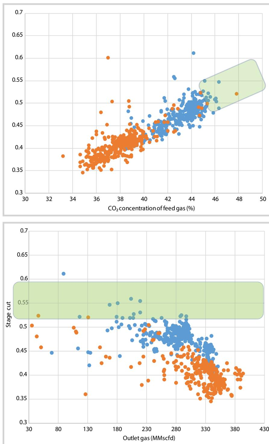
Figure 8. Depends of outlet gas on CO<sub>2</sub> concentration of feed gas.
