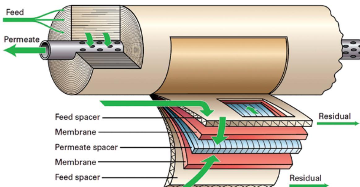
\*Two membrane sheets with permeate spacer between: leaves are separated by feed spacers and wrapped around a permeate tube facing it with three open ends.
