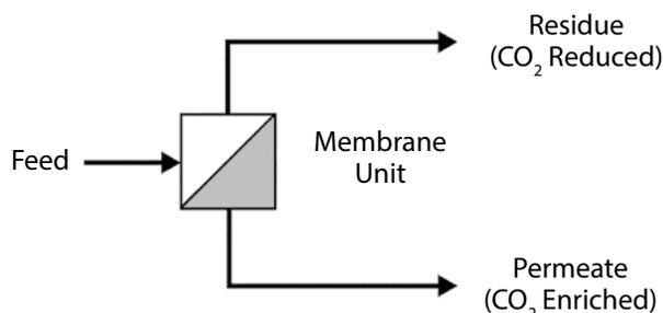
Figure 3. Single-stage flow scheme
