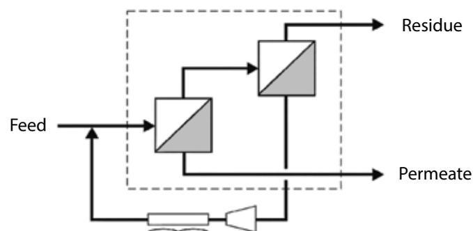
Figure 4. Dual-stage flow scheme.
