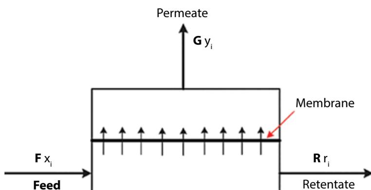
Figure 1. Schematic illustration of membrane separation process.
